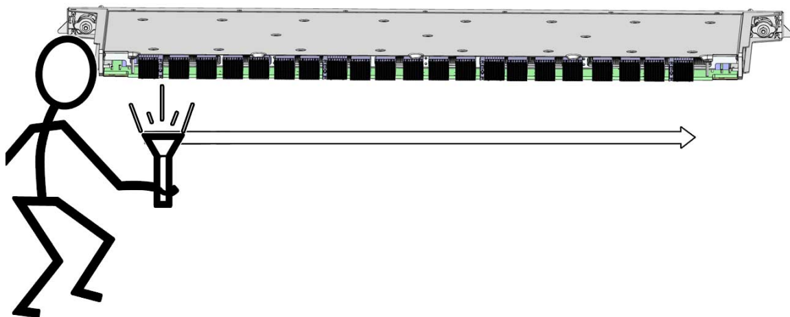
FIGURE 7-1 Inspecting Line Card Connectors
